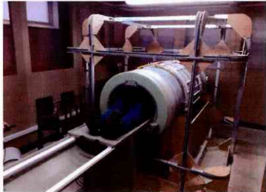
Figure 1: Photograph of the 0.2 T FFC-MRI scanner and Earth's-field compensation coils.
